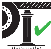
Hard Level Surface e.g. concrete
