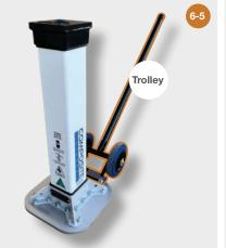
The placement trolley specifically designed to mount onto 35t type 2 & 3; jack stands to manoeuvre them in and out of position. It has a extendable handle of 1.2 to 2m to keep technicians out of the line of fire and reduces the risk of personal injury that is related to the manual handling of jack stands.
