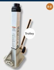
• The placement trolley specifically designed to mount onto type 2, 3 & DZ; 50t jack stands to manoeuvre them in and out of position. It has a extendable handle of 1.2 to 2m to keep technicians out of the line of fire and reduces the risk of personal injury that is related to the manual handling of jack stands.
