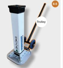
• The placement trolley specifically designed to mount onto 35t type 2 & 3; jack stands to manoeuvre them in and out of position. It has a extendable handle of 1.2 to 2m to keep technicians out of the line of fire and reduces the risk of personal injury that is related to the manual handling of jack stands.
