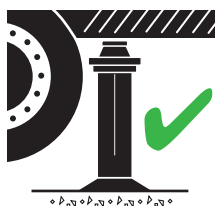
Hard Level Surface e.g. concrete
